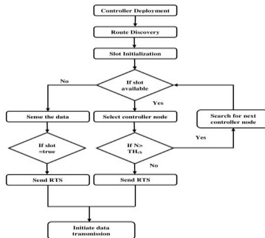
Fig. 1. Work flow of proposed PCS-SRD approach.
