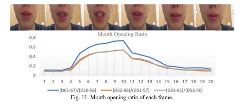
In Fig. 11, the curve from left to right is the process of speaking, and it shows the ratio of the mouth opening we measured. When the mouth opening ratio is greater than a certain threshold, then it can be determined that the person is opening the mouth and talk. After the testing, the threshold is preferably about 0.09, as shown in Fig. 11. The algorithm
