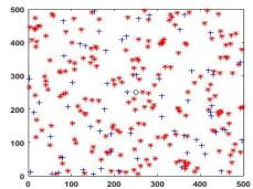
Fig. 2. Deployment of sensors in the wireless sensor network with base-station at the center.
