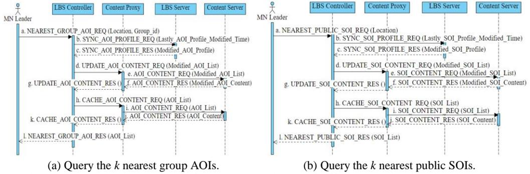
Fig. 6. The message flow diagrams for the control schemes of different querying functions in the narrator mode, part B.
