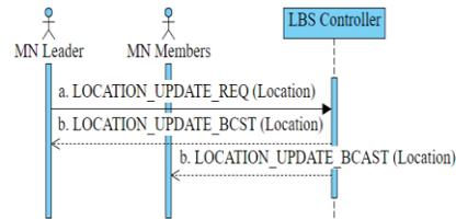
Fig. 4. The message flow diagram of the control scheme for the positioning function in the narrator mode.
