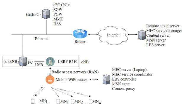
Fig. 12. The networking configuration of the experiment.
