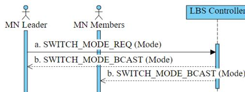
Fig. 9. The message flow diagram of the control scheme for the mode-switching function.
