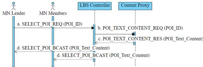
Fig. 7. The message flow diagram of the control scheme for the selecting POI function in the narrator mode.
