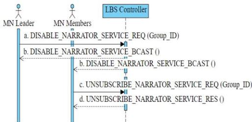
Fig. 3. The message flow diagram of the control scheme for the disabling service function and the unsubscribing service function.
