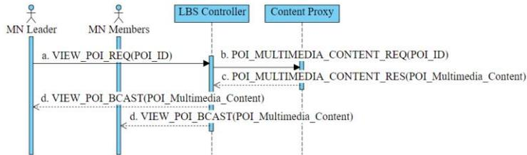
Fig. 8. The message flow diagram of the control scheme for the viewing function in the narrator mode.
