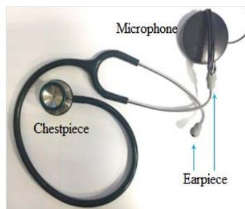
Fig. 1. Bronchial breath sound measurement tools: stethoscope and microphone.
