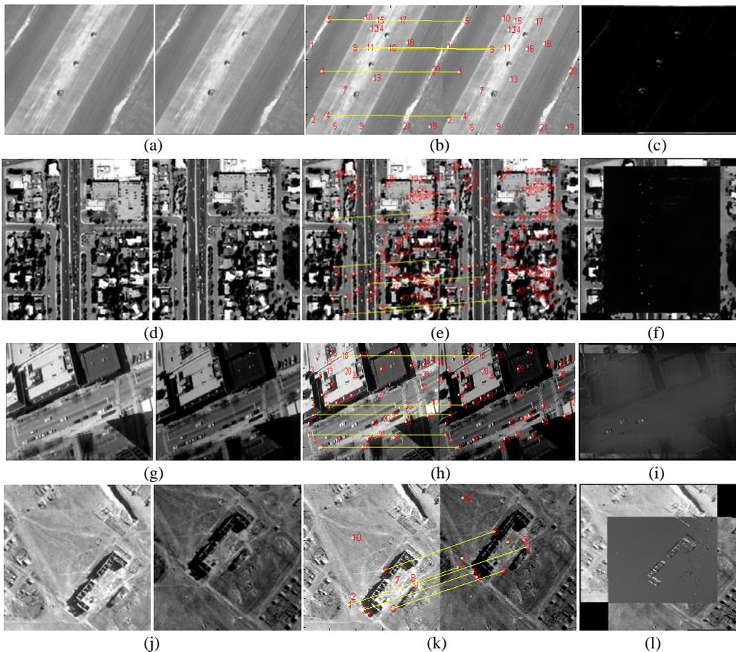
Fig. 9. Absolute differences registration results of planar background scene, complex urban scene and illumination change; (a) Two aerial images of planar background scene; (d) Two aerial images of complex urban scene; (g) and (j) Two aerial images of illumination change; (b), (e), (h) and (k) The matching points pair; (c), (f), (i) and (l) Registration.
