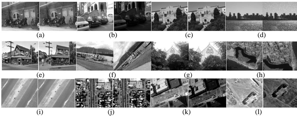
Fig. 4. Test image pairs taken from the textured and structured scenes under photometric or geometric transformation; (a) Bikes(blur); (b) Leuven (lighting); (c) UBC (JPEG); (d) Sea (noise); (e) Graffito (viewpoint); (f) Boat (rotation); (g) Church (scale); (h)-(l) Aerial photography.
