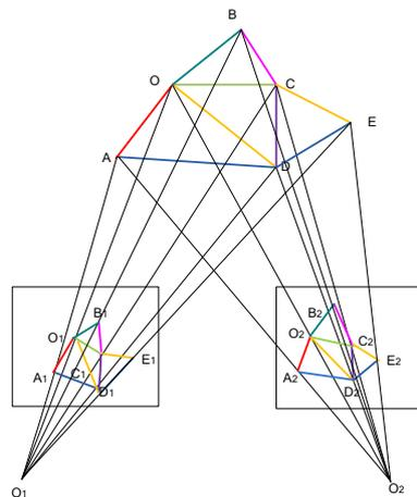
Fig. 2. The cross-ratio invariance of the four lines.
