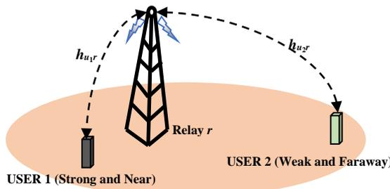
Fig. 1. Uplink phase and downlink phase of two-way relay based NOMA system.
