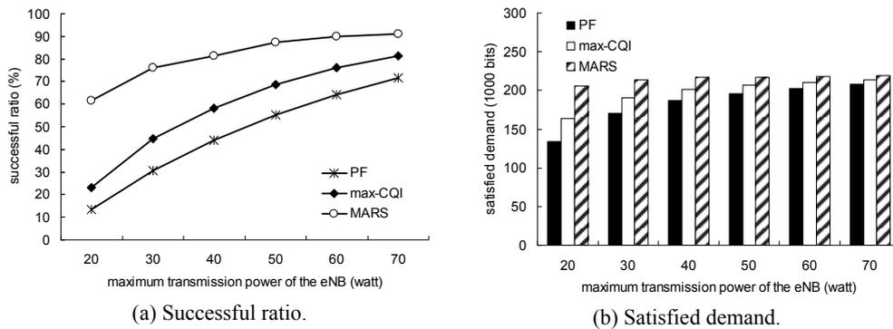
Fig. 6. Comparison on the scheduling results under different  $P_{max}$  power.
