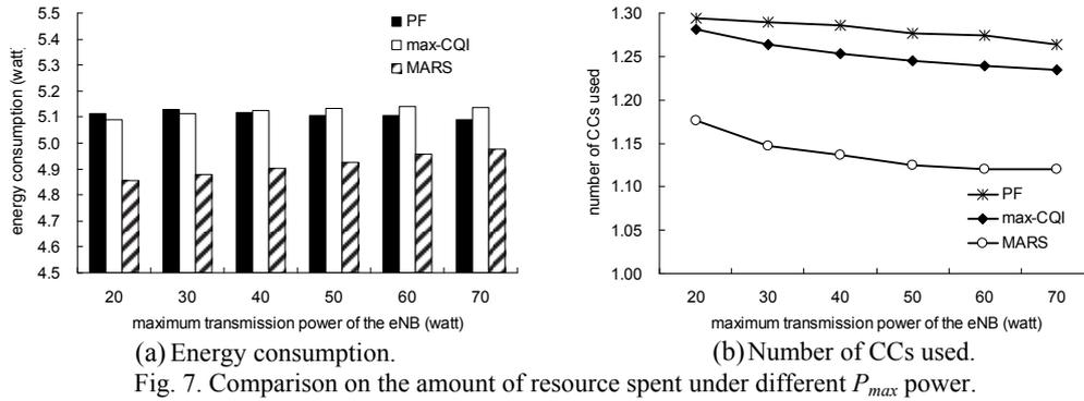
Fig. 7. Comparison on the amount of resource spent under different  $P_{max}$  power.
