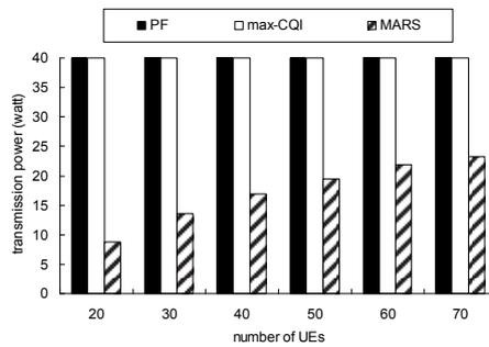
Fig. 4. Comparison on the eNB's transmission power under different number of UEs.
