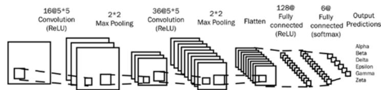
Fig. 9. The CNN architecture composed of two convolutional layers and two fully-connected layers.
