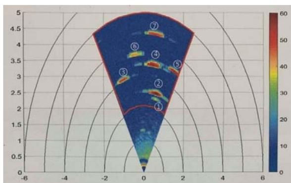
Fig. 3. The R-A map. It shows the response from the target echoes. It can be seen from the figure that there are seven ship targets. From this figure, we can see the intensity of the echo reflection of each ship target and its two-dimensional range.
