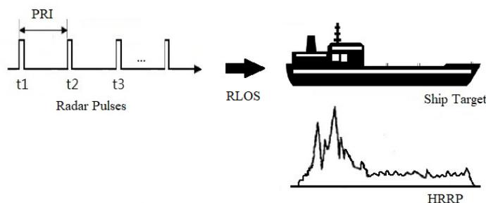
Fig. 1. Schematic diagram of radar HRRP for ship targets.
