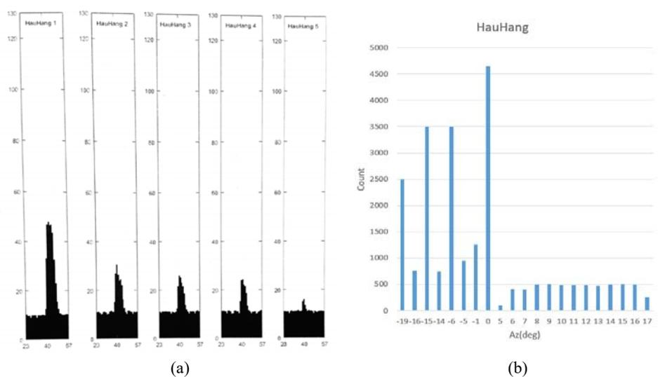
Fig. 5. An example: the HRRPs of the same ship collected at different azimuth angles and its histogram; (a) shows the HRRPs of the same ship named HuaHang collected at different azimuth angles; (b) exhibits the histogram of HuaHang's HRRPs collected at different azimuth angles.
