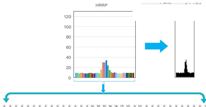
Fig. 8. Schematic diagram of the two-dimensional binary-map HRRP data format.
