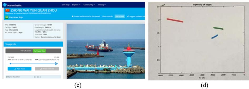
Fig. 4. Some examples of AIS information and trajectories of the collected ships; (a) and (c) show the AIS information of two ships; (b) and (d) show the trajectories of the two ships shown in (a) and (c), respectively. Each different color trajectory represents a different continuous data collected. These data can indicate that the ship data collected are diverse, including different ranges and azimuths.
