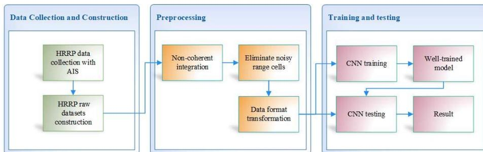
Fig. 2. The function blocks of the proposed approach.
