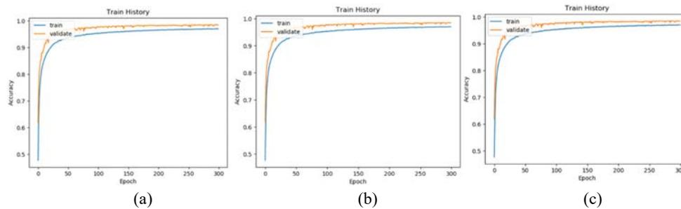
Fig. 12. Recognition accuracy curve of training and testing set for three data formats: (a) one-dimensional HRRP data format; (b) two-dimensional gray-scale HRRP data format; and (c) two-dimensional binary-map HRRP data format.
