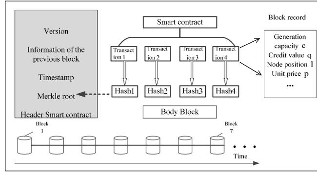
Fig. 2. Data structure of the CIB.
