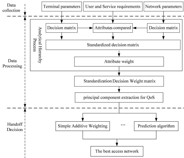
Fig. 2. The vertical handoff algorithm with ensuring QoS.
