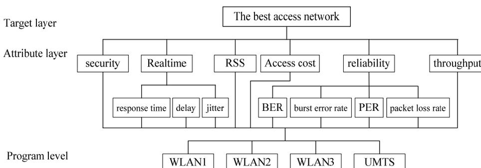
Fig. 3. The attribute hierarchical structure tree.
