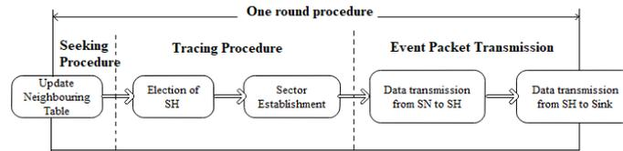
Fig. 9. One round procedure of the sectoring scheme using the CSO technique.
