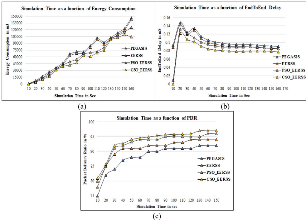
Fig. 11. (a) Energy consumption as a function of ST; (b) Packet delivery ratio as a function of ST; (c) Average end to end delay as a function of ST.
