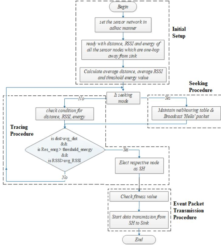
Fig. 8. Flowchart of execution of the sectoring scheme using CSO.
