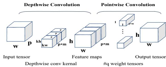
Fig. 6. The schematic overview of DSC.
