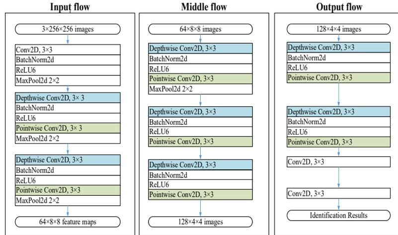
Fig. 8. The proposed MobileNet-based CNN structure.
