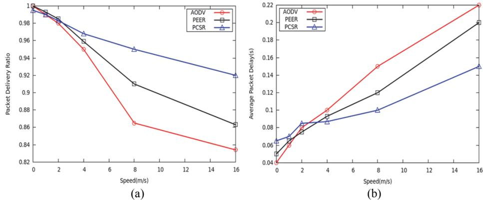
Fig. 4. Results of (a) packet delivery ratio; (b) average packet delay.
