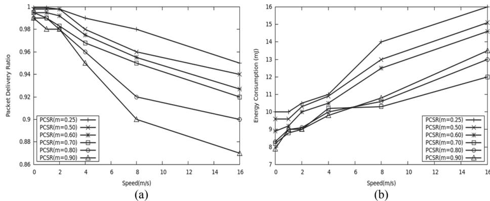
Fig. 3. Impacts of different values of  $m$  on (a) packet delivery ratio; (b) energy consumption.
