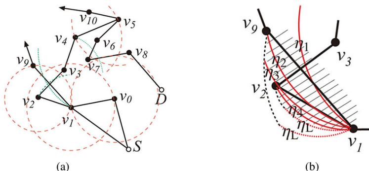
Fig. 2. (a) Recovery mode starts at  $v_0$  for a packet from  $S$  to  $D$ . Node  $v_1$  performs eSW to locate node  $v_2$ , resolving the issue of crossing edges  $v_1v_9$  and  $v_2v_3$ . Node  $v_5$  performs  $\alpha$ -CO to locate next relay  $v_6$  that should have been selected by but was hidden from node  $v_4$  previously; (b) Enhanced sweep (eSW) searches to locate  $v_2$  are highlighted. The eSW has been invoked twice here.
