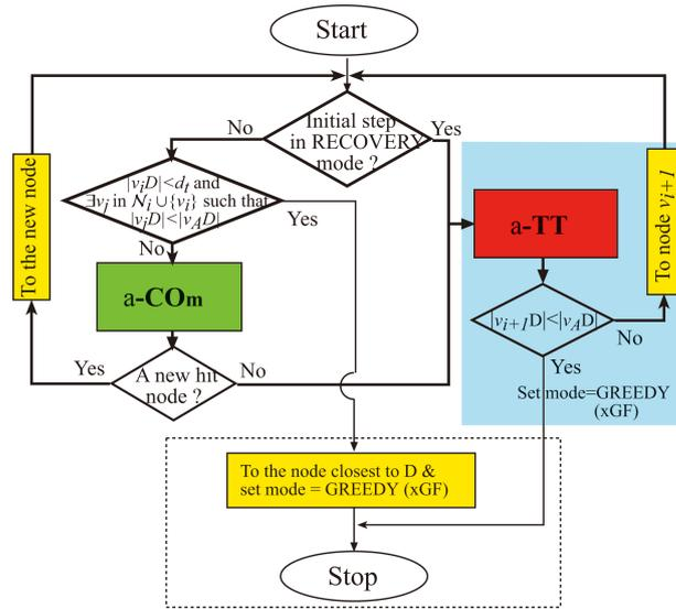
Fig. 4. The flow chart of recovery scheme involving  $\alpha$ -CO<sub>m</sub>TT and operation mode change to GF. The way to terminate routing is not shown.
