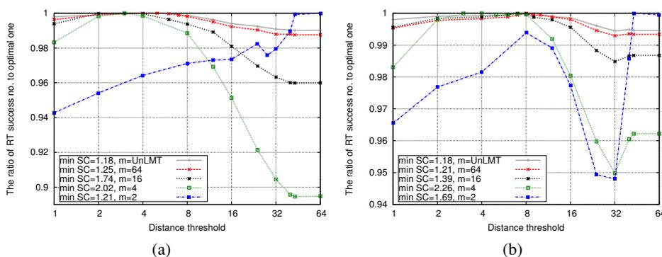
Fig. 10. The ratio of routing success performance to optimal achievable one versus distance threshold  $d_t$  for path loss exponent 4 and networks (a) with no artificial void and 4200 nodes and (b) with two artificial voids and 3840 nodes. Optimal minimum SC size  $\eta_L$  for each  $m$  is employed. UnLMT indicates  $\infty$ .
