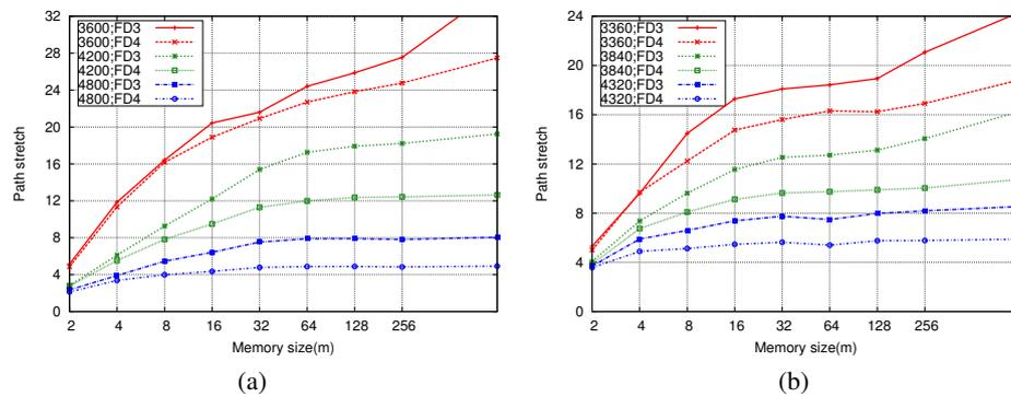
Fig. 8. Average SD-path hop count stretch versus memory length ( $m$ ) for networks (a) without artificial voids and (b) with two artificial voids.
