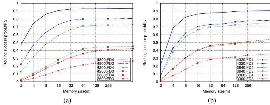
Fig. 7. The probability of successful routing from S to D versus memory length ( $m$ ) for networks (a) without artificial voids and (b) with two artificial voids.
