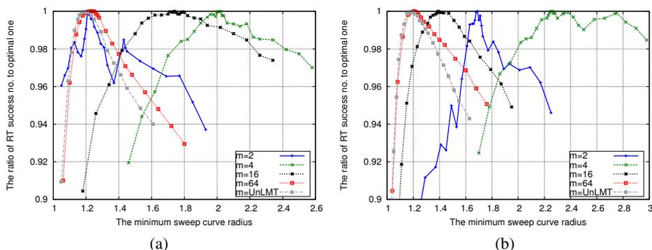
Fig. 9. The ratio of optimal routing success performance under a given minimum SC size  $\eta_L$  to the global optimal one versus  $\eta_L$ , for path loss exponent 4 and networks (a) with no artificial void and 4200 nodes and (b) with two artificial voids and 3840 nodes. Results are optimized with regard to  $d_t$ . UnLMT indicates  $\infty$ .
