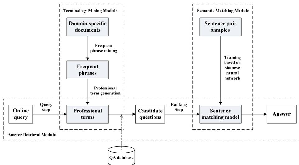
Fig. 1. The architecture of the proposed domain-specific non-factoid QAS.
