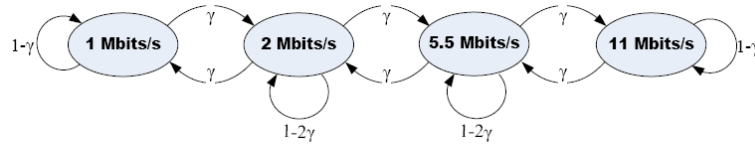
Fig. 15. The state transition diagram of QSTAs' transmission rates.
