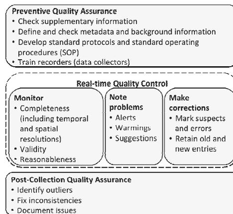
Fig. 6. Data quality assurance (QA) and quality control (QC) for disaster data recording.
