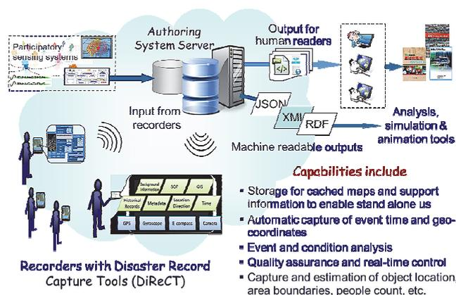
Fig. 2. DiSRC system framework and overview.
