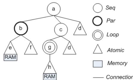
Fig. 4. The design hierarchy of a set of connected HFSMs.
