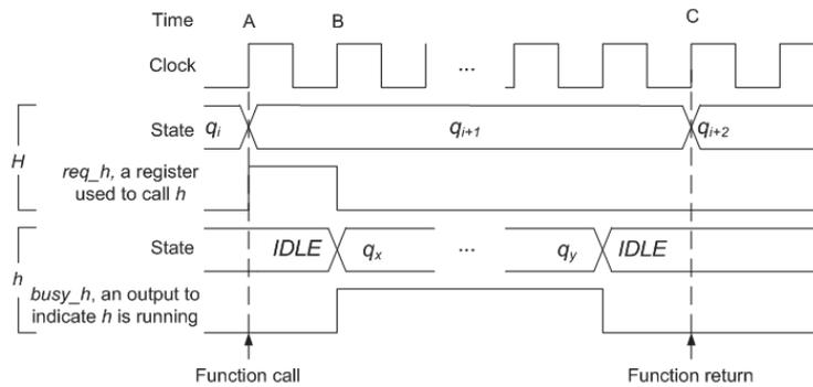
Fig. 3. The waveform of the communication protocol between HFSM  $H$  and its child  $h$ .
