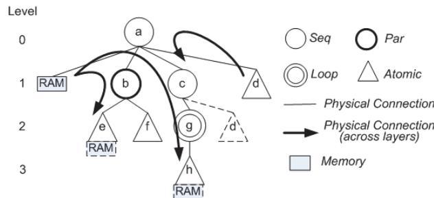
Fig. 5. The physical connections of the hardware blocks represented by distinct HFSMs.
