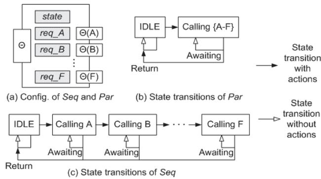
Fig. 2. (a) The configuration of the templates of *Seq* and *Par*; we have registers  $req_x$  connected to  $\Theta(x)$  used to call block  $x$ , where  $x \in \{A-F\}$ ; (b-c) Their state transitions with or without actions.
