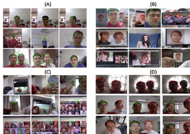
Fig. 7. Snapshots of testing results in (a) true positive group; (b) true negative group; (c) miss detection group; (d) false alarm group.
