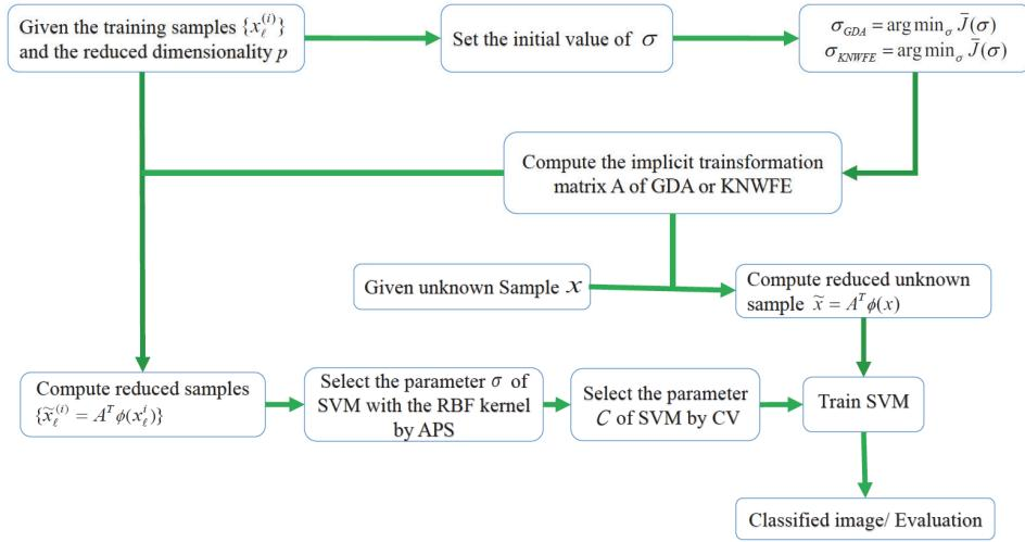
Fig. 1. Proposed kernel-based classification scheme, GDA+SVM or KNWFE+SVM with APS.
