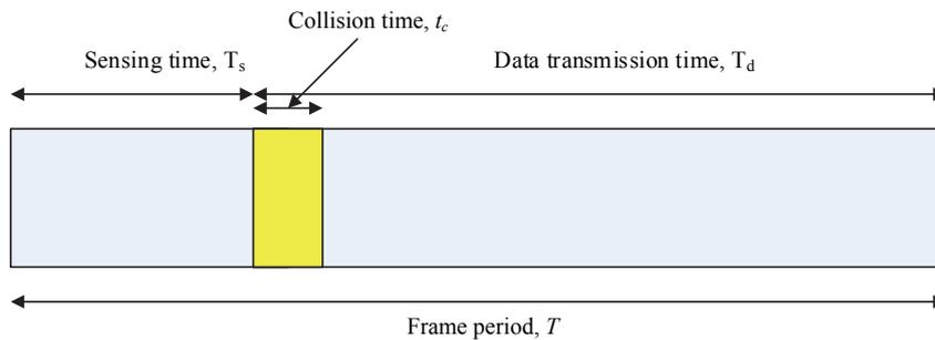
Fig. 2. Time frame structure of cognitive radio network.
