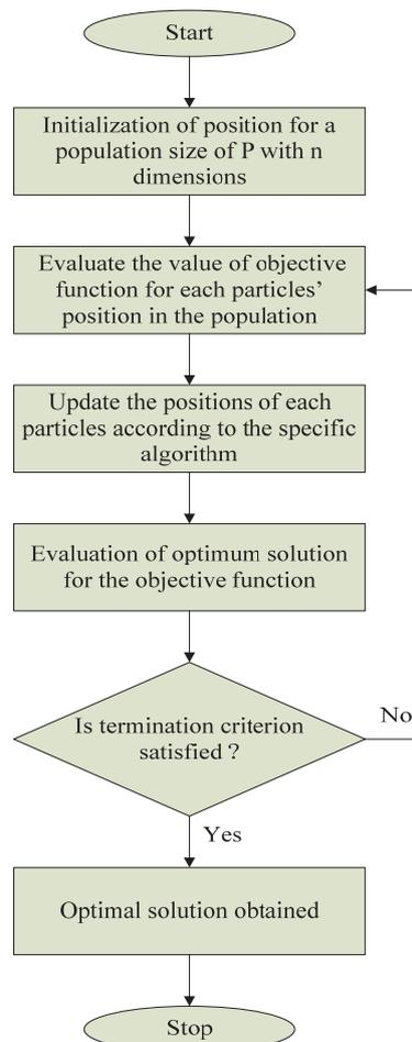
Fig. 4. Flowchart of the optimization process.
