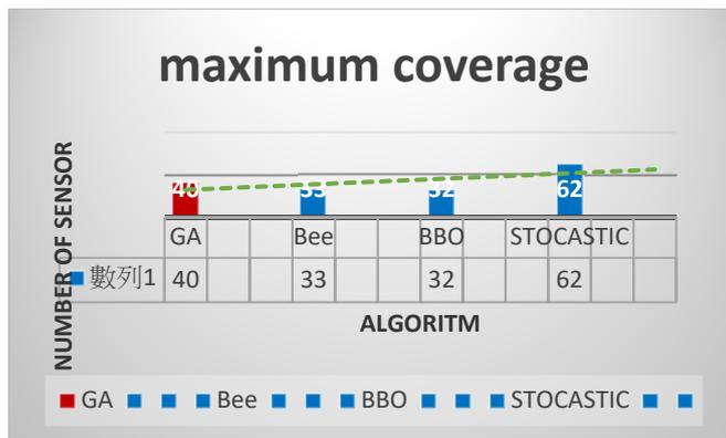
Diagram 2: The number of needed sensors for 100% coverage.
