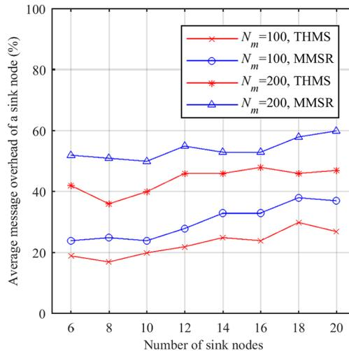
Fig. 9. Comparison of message overhead.
