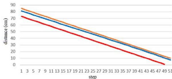
Fig. 10. The distance calculated by the inner ellipse and the circumscribed ellipse methods. The orange line represents the actual distance of the two links, the blue line represents the distance calculated by the inner ellipse method, and the red line represents the distance calculated by the circumscribed ellipse.
