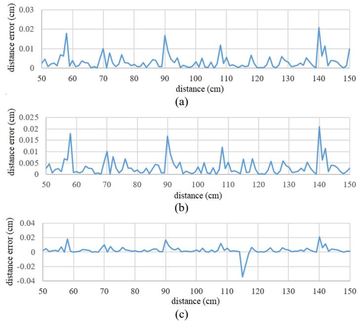
Fig. 6. The distance error between polynomial function and real curve; (a) Quadratic polynomial function; (b) Cubic polynomial function; (c) Quadric polynomial function.
