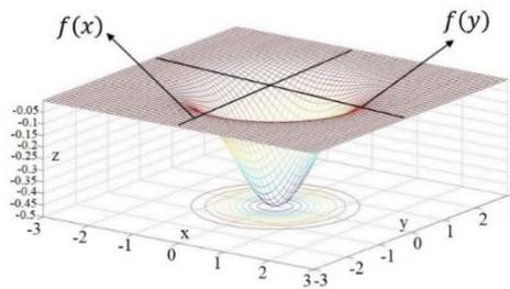
Fig. 3. Multiplication of two one-dimensional Gaussian functions.
