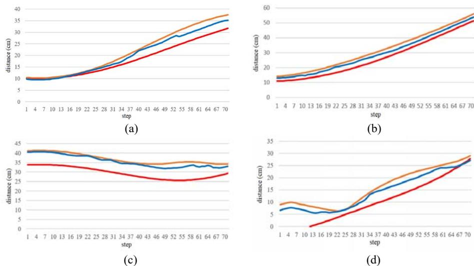
Fig. 14. The distance changes between the obstacle and the link; (a) The influence of the bottom obstacle on the first link; (b) The influence of the bottom obstacle on the second link; (c) The influence of the top obstacle on the first link; (d) The influence of the top obstacle on the second link.
