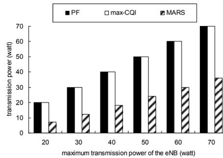
Fig. 8. Comparison on the eNB's transmission power under different  $P_{max}$  power.
