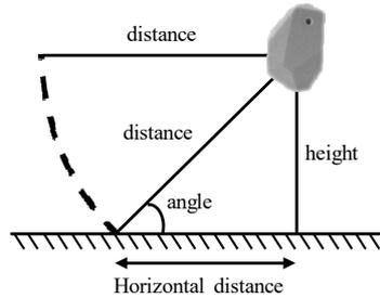
Fig. 1. The conversion between the measured distance and horizontal distance.
