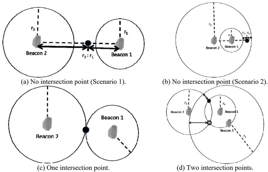
Fig. 2. Schematic of the intersection points of two circles.
