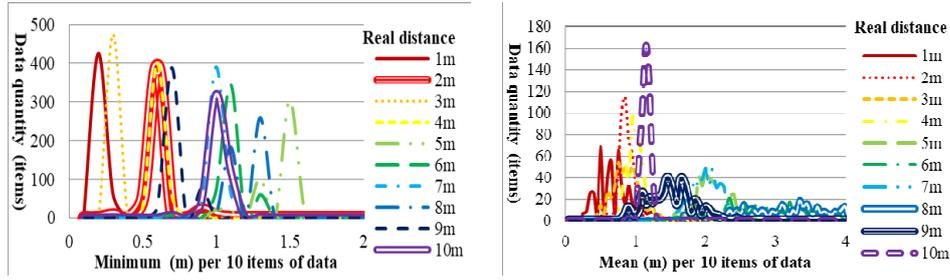
Fig. 5. Various statistics for data measured at various actual distances (1–10 m) obtained from every 10 items of continuous data.
