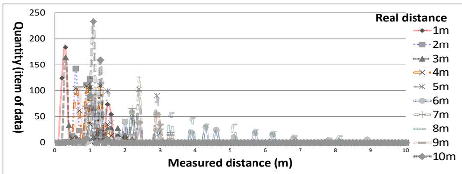
Fig. 4. Distribution of measured distances from ten real distances (with transmission powers 4dBm and transmission periods 100m).
