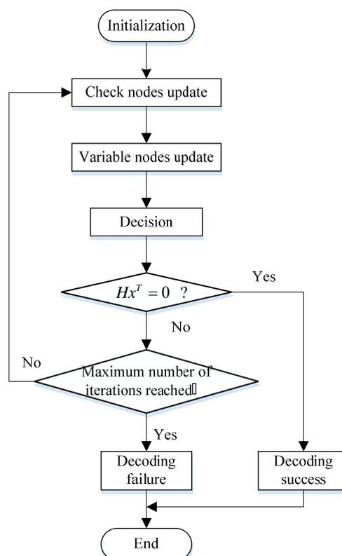
Fig. 2. Flow diagram of BP algorithm.
