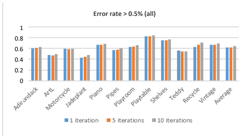
Fig. 18. Error rates with error > 5% for all pixels achieved by the proposed recursive refinements with 1, 5 and 10 iterations.
