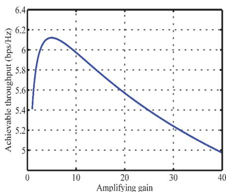
Fig. 5. Average achievable throughput versus amplifying gain of the relay.
