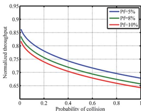
Fig. 7. Normalized throughput of the network versus probability of collision.
