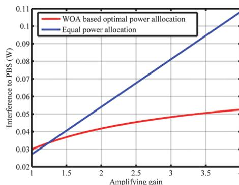
Fig. 10. Interference to PBS versus amplifying gain of the relay.
