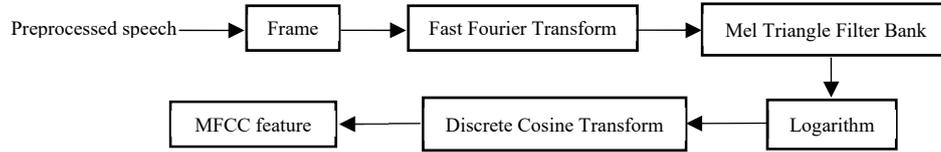
Fig. 1. The process of traditional MFCC feature extraction.
