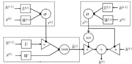
Fig. 6. The data flow in GRU.
