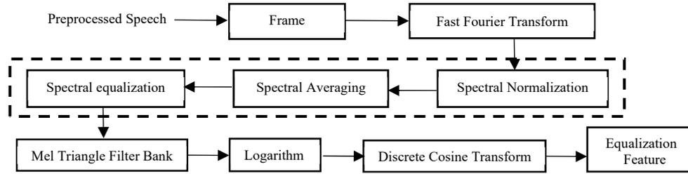
Fig. 2. The process of equalization feature extraction.
