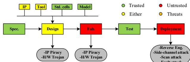
Fig. 1. Security threats at different stages of SoC development and deployment cycle [3].
