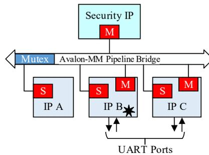
Fig. 18. Block diagram of a SoC benchmark system instance.
