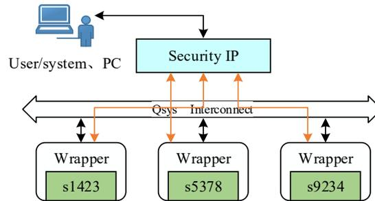
Fig. 11. Block diagram of our SoC benchmark system.
