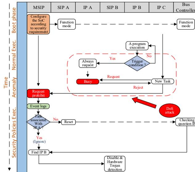
Fig. 10. Operation flow of the proposed solution for preventing DoS attacks.
