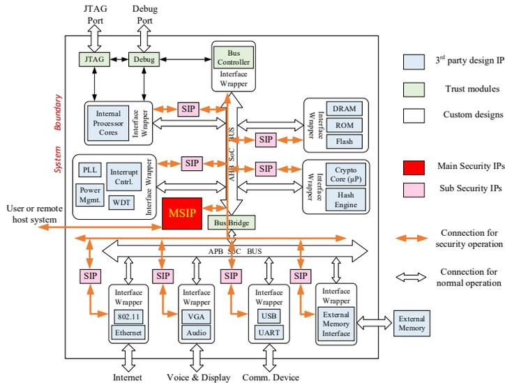
Fig. 2. Block diagram of the proposed MSIPS architecture in a generic SoC.
