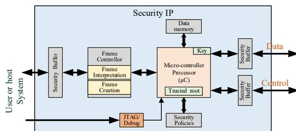
Fig. 5. Block diagram of security IP module.
