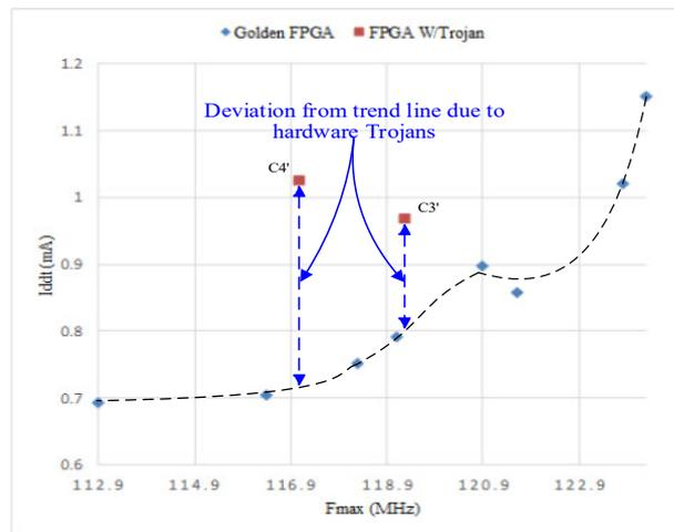
Fig. 14. Variation curve of the slope values ( $I_{ddt}$  vs.  $F_{max}$ ) acquired on 10 FPGA chips using multi-parameter based Trojan detection technique.
