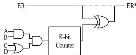
Fig. 12. A generic hardware Trojan circuits implanted in SoC benchmark system.
