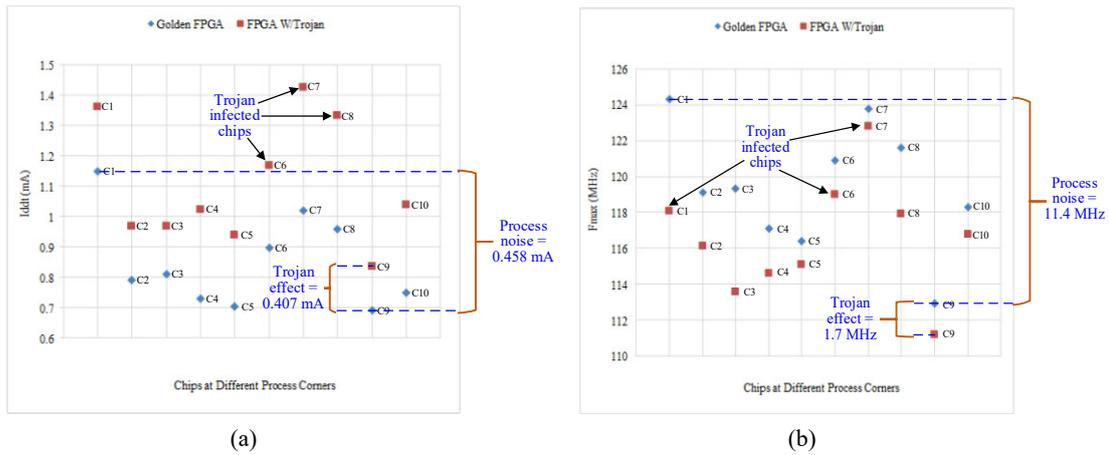
Fig. 13. The single-parameter based Trojan detection results on FPGA; (a) Measurement of average  $I_{ddt}$  values only at 10 random process corners; (b) Corresponding  $F_{max}$  values.
