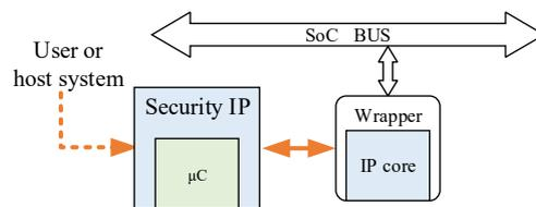
Fig. 4. Block diagram of Security IPs connected to other individual IPs.
