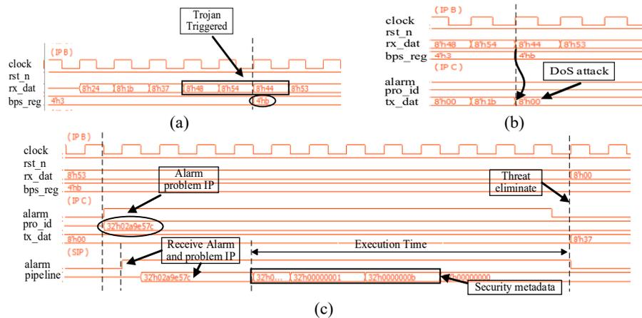
Fig. 19. Simulation results of security IP against DoS attacks; (a) Trigger the Trojan instance; (b) IP C fails to read IP A; (c) Alarm threats and eliminate them.
