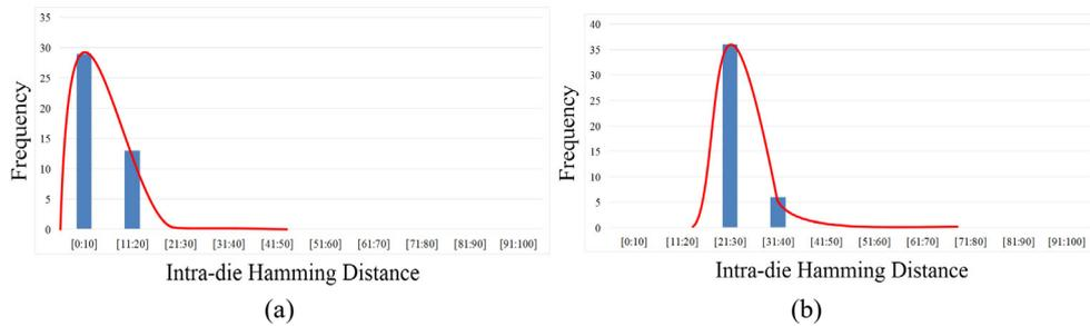
Fig. 17. The reliability distribution among a variety of operating temperature; (a) Intra-die HDs of the CRO-PUFs; (b) Intra-die HDs of the common RO-PUFs.
