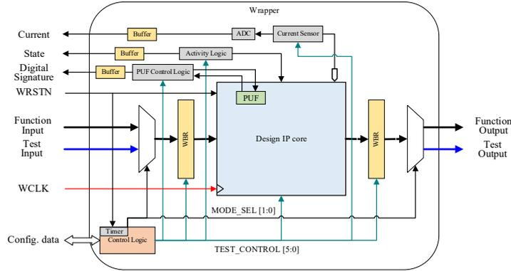
Fig. 7. Block diagram of security IP module.
