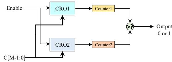
Fig. 9. A general structure of CRO-PUF module.
