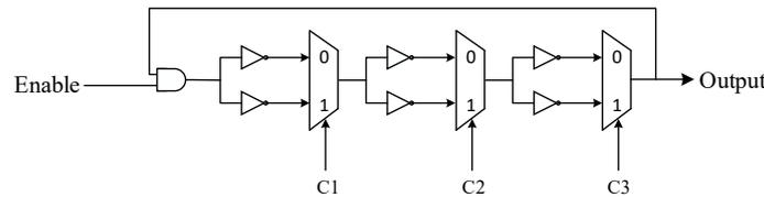
Fig. 8. The basic structure of a CRO circuit.
