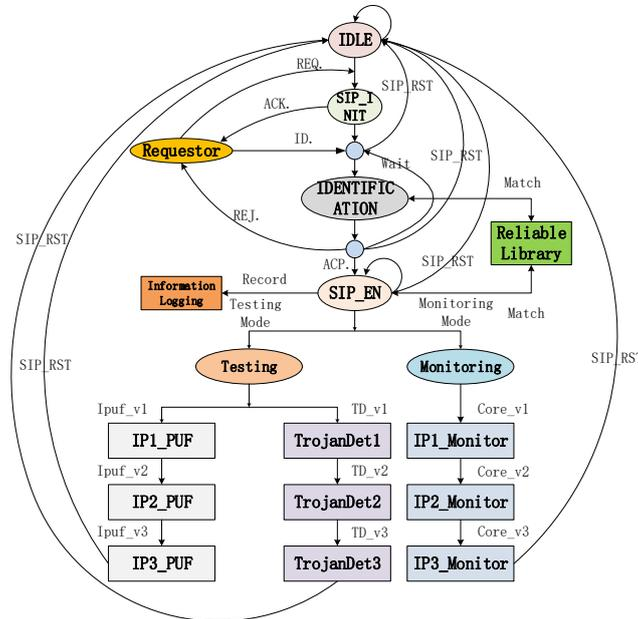
Fig. 3. State transition diagram of the sub security IP module.
