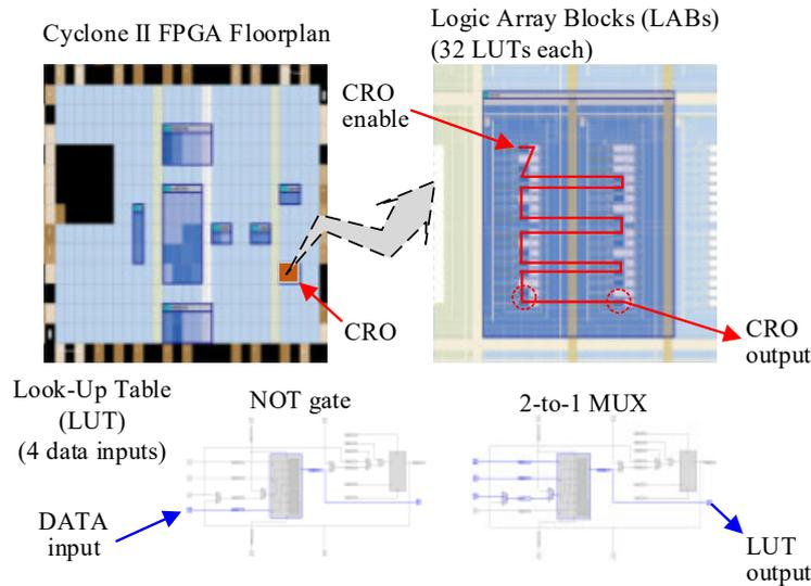
Fig. 15. Generic LABs with a CRO circuit implemented on FPGA.
