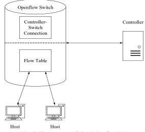
Fig. 9. The structure of simulation for SDN.
