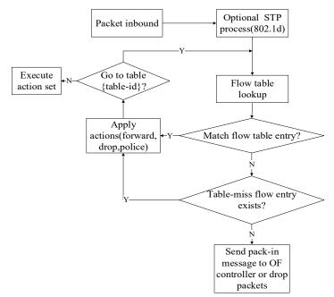
Fig. 2. Handling a packet flow in OpenFlow switch.
