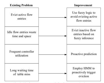
Fig. 3. The improvements made by the proposed scheme.
