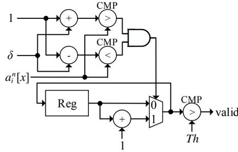
Fig. 7. Hardware architecture of the SVSEE checker.
