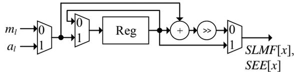
Fig. 5. Hardware architecture of the interpolating module.
