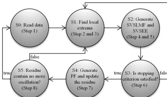
Fig. 1. State diagram of the LMD hardware.
