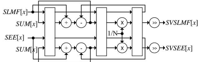
Fig. 6. Hardware architecture of the smoothing module.
