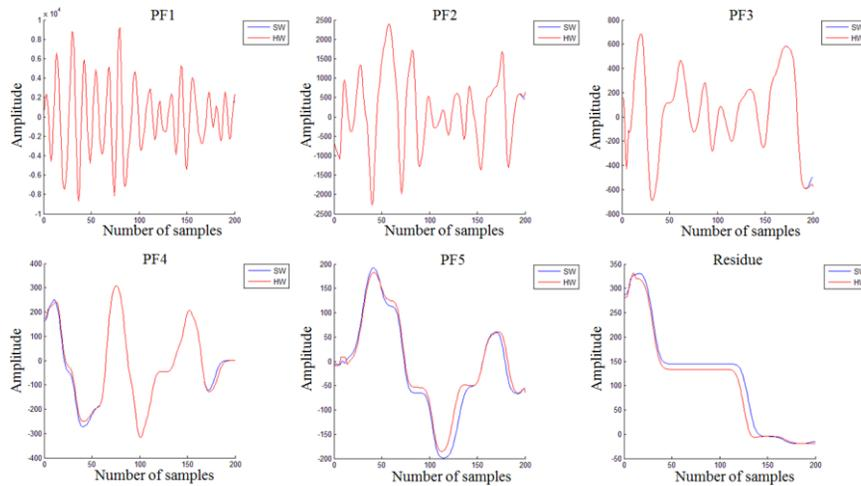
Fig. 12. Comparison of applying LMD to an ECG signal when using a software solution and the proposed hardware solution with 24-bit precision.
