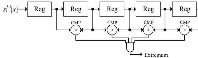
Fig. 3. Hardware architecture of the extrema extractor.
