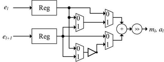
Fig. 4. Hardware architecture of the feature generator.
