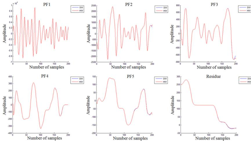
Fig. 11. Comparison of applying LMD to an ECG signal when using a software solution and the proposed hardware solution with 48-bit precision.
