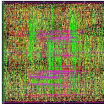
Fig. 10. Layout of the proposed 48-bit design developed using the TSMC 0.18- $\mu\text{m}$  cell library.
