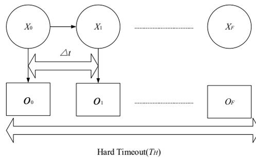
Fig. 6. The structure of the proposed HMM.
