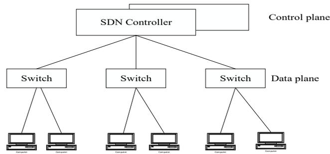
Fig. 1. The structure of SDN.
