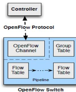
Fig. 1. The OpenFlow Switch architecture.
