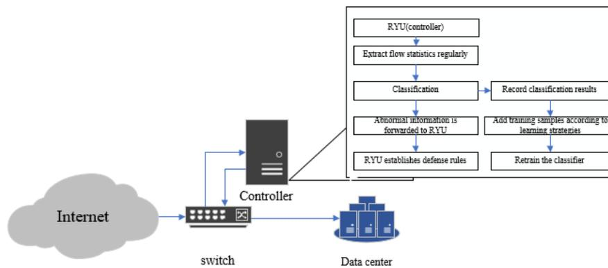
Fig. 2. Our SDN intrusion detection architecture.
