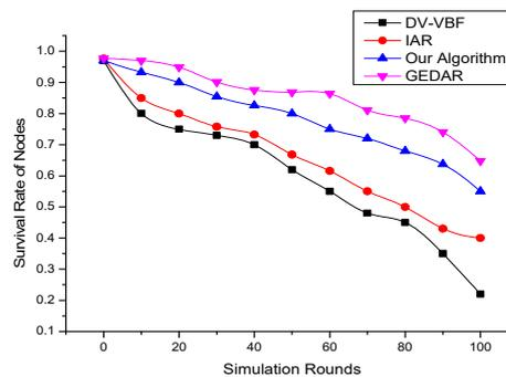
Fig. 5. The comparison of network lifetime.
