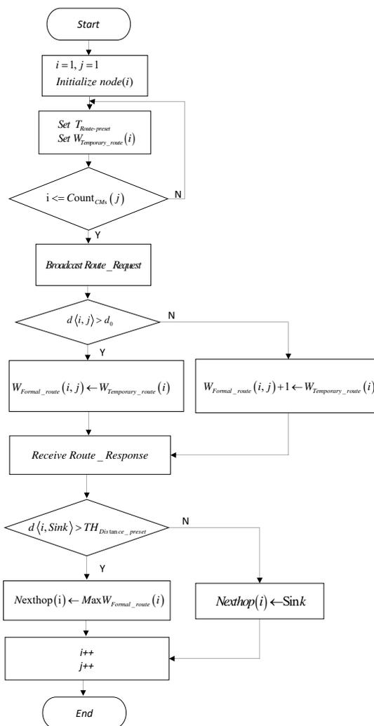
Fig. 3. The data transmission phase.
