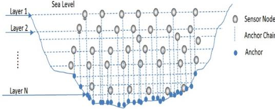
Fig. 1. The hierarchical network model.
