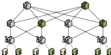
Fig. 3. A WDC of Clos architecture with driver nodes painted green.
