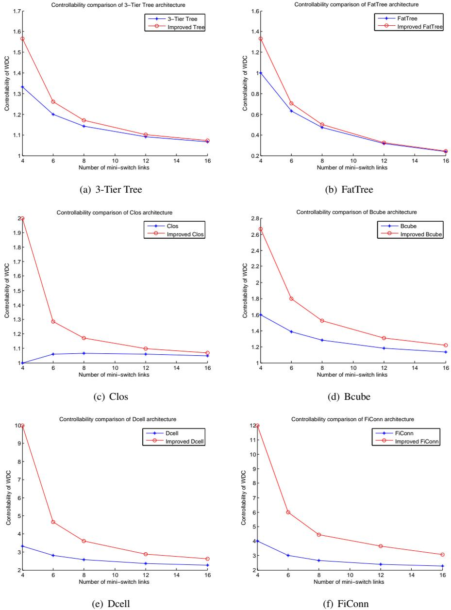
Fig. 8. Experimental results of controllability adjustment on mainstream WDC architectures. The X-axis is  $d$ , the number of links of switches in the WDCs, the Y-axis is  $n_D$ , the corresponding controllability. The blue lines marked by '\*' stand for the original controllability of WDCs, while the red lines marked by 'o' shows the improved results. Note that the scale ranges of Y-axis vary in different subfigures.
