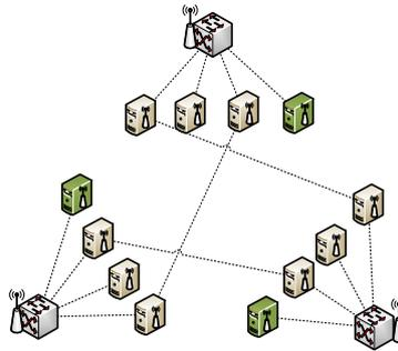
Fig. 6. A WDC of FiConn architecture with driver nodes painted green.
