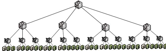
Fig. 1. A WDC of Three-Tier architecture with driver nodes painted green.
