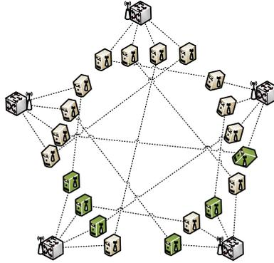
Fig. 5. A WDC of Dcell architecture with driver nodes painted green.
