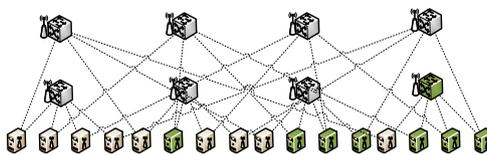
Fig. 4. A WDC of Bcube architecture with driver nodes painted green.
