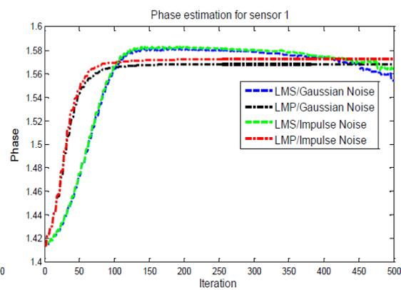
Fig. 12. Convergence diagram and estimation of the first sensor phase locally.
