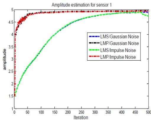
Fig. 11. Convergence diagram and estimation of the first sensor domain.
