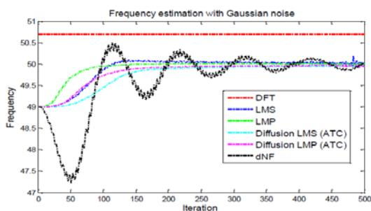
Fig. 3. Convergence diagram and estimation in Gaussian noise mode.
