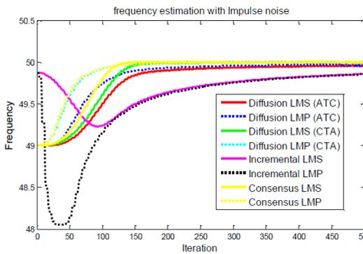
Fig. 9. Convergence diagram and estimation of distributed frequency with impulse noise.
