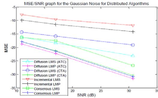
Fig. 8. MSE chart in terms of SNR distributed methods in Gaussian noise mode.
