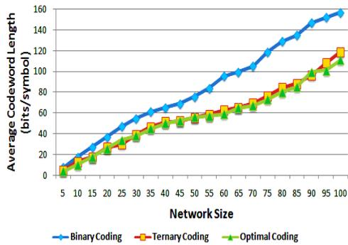
Fig. 6. Comparison of average codeword length for binary, ternary and optimal Huffman coding schemes.
