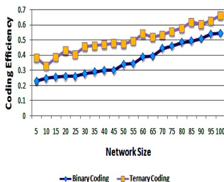
Fig. 5. Coding efficiency for binary and ternary coding schemes with varying network sizes.
