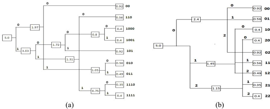
Fig. 3. Huffman (a) binary and (b) ternary coding trees corresponding to the transmission attempt probabilities of different nodes in the sample ad-hoc network.
