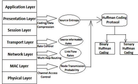
Fig. 1. Proposed cross-layer design architecture implemented with Huffman coding protocol.
