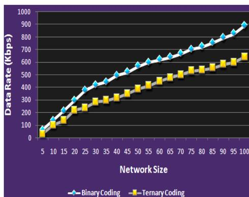
Fig. 4. Maximal data rate attained for binary and ternary coding with different network sizes.
