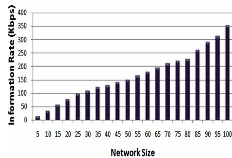
Fig. 9. Minimal required information rate for different network sizes.
