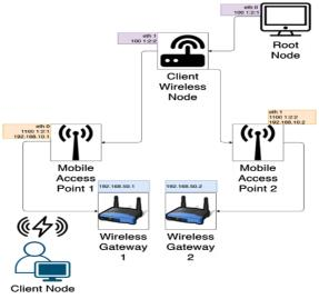
Fig. 4. WPIv6 network experimental configuration.
