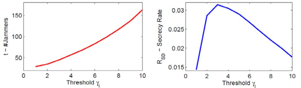
Fig. 7. Smart jamming; (a) Number of jammers vs the threshold  $\gamma_i$ ; (b) The secrecy rate  $R_{SD}$  that can be achieved. Here  $R = 100\text{m}$ ,  $\gamma_e = -3\text{dB}$ ,  $\lambda_E = 0.00002$ ,  $\varepsilon_S = 90\text{dB}$ , and the secrecy outage probability  $P_{SO} < 0.1$ .
