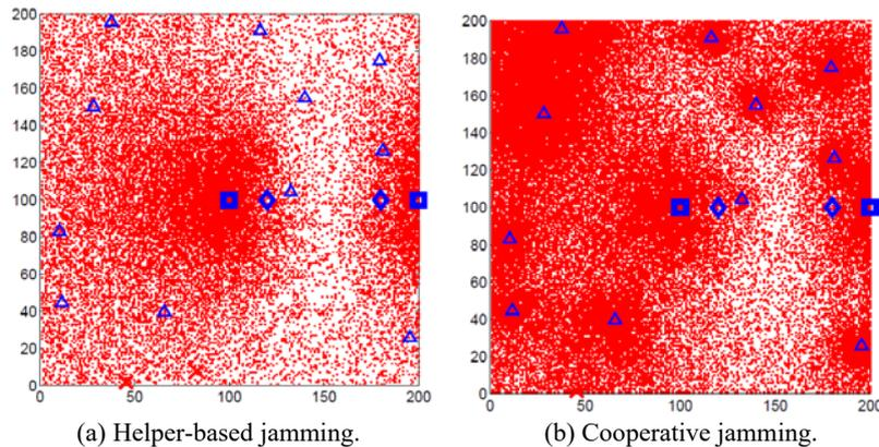
Fig. 4. Examples of jamming strategies in fading channels.  $S$  is located at (100, 100),  $D$  at (200, 100),  $\Delta$  denotes jammer,  $\diamond$  denote helper, and the red area represents the jamming region. Here  $P_S/N_0 = 90\text{dB}$ ,  $\lambda = 0.0003$ ,  $\lambda_E = 0.00005$ ,  $\alpha = 3$ ,  $R = 100\text{m}$ ,  $\gamma_I = 10\text{dB}$ , and  $\gamma_e = -10\text{dB}$ . All links experience unit mean Rayleigh fading.
