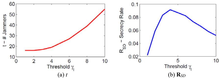
Fig. 8. Cooperative jamming. (a) Number of jammers vs the threshold  $\gamma$ ; (b) The secrecy rate  $\mathbf{R}_{SD}$  that can be achieved. Here  $R = 100\text{m}$ ,  $\gamma_e = -3\text{dB}$ ,  $\lambda_E = 0.00002$ ,  $\varepsilon_S = 90\text{dB}$ , and the secrecy outage probability  $P_{SO} < 0.1$ .
