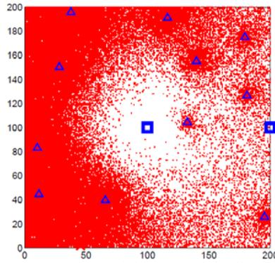
Fig. 2. Example of smart jamming strategy in fading channels.  $S$  is located at  $(100, 100)$ ,  $D$  at  $(200, 100)$ ,  $\Delta$  denotes jammer, the red area represents the jamming region. Here  $P_S/N_0 = 90\text{dB}$ ,  $\lambda = 0.0003$ ,  $\lambda_E = 0.00005$ ,  $\alpha = 3$ ,  $R = 100\text{m}$ ,  $\gamma = 10\text{dB}$ , and  $\gamma_e = -10\text{dB}$ . All links experience unit mean Rayleigh fading.
