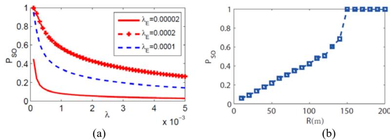
Fig. 5. Secrecy outage probability vs. (a)  $\lambda$  ( $R = 50\text{m}$ ), and (b)  $R$  ( $\lambda = 0.0001$ ,  $\lambda_E = 0.00002$ ). Here  $\varepsilon_S = 97\text{dB}$ ,  $\gamma_l = 10\text{dB}$ , and  $\gamma_e = -3\text{dB}$ .
