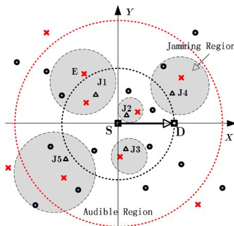
Fig. 1. The network model.  $\times$ ,  $\Delta$ , and  $\circ$  denote eavesdropper, jammer, and legitimate nodes, respectively. The shaded disc is the jamming region of a jammer. Any eavesdropper  $E$  located within a jamming region will have its  $\gamma_{SE} < \gamma_e$ .
