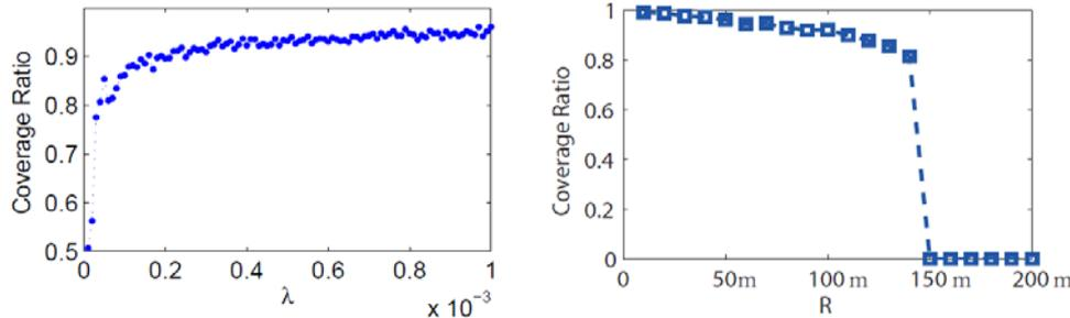
Fig. 6. Coverage ratio vs. (a)  $\lambda$  ( $R = 80\text{m}$ ,  $\varepsilon_S = 92\text{dB}$ ), and (b)  $R$  ( $\lambda = 0.0001$ ,  $\varepsilon_S = 97\text{dB}$ ). Here  $\gamma = 10\text{dB}$ ,  $\gamma_e = -3\text{dB}$ .
