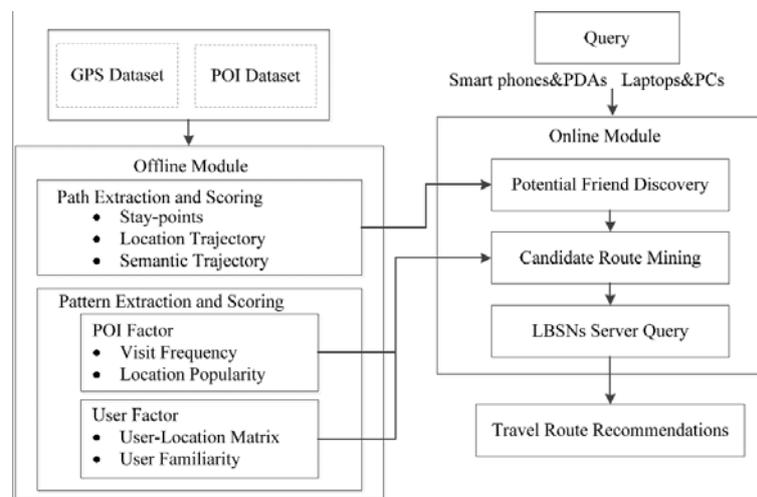
Fig. 2. The framework and flow of data processing within *PP-TRR*.
