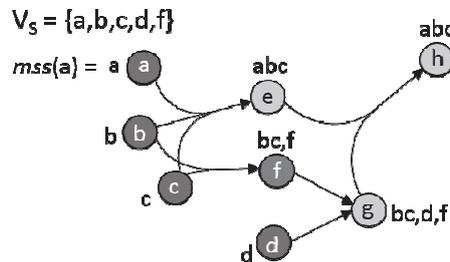
Fig. 5. An example of minimal source sets.  $abc$  is a shorthand notation of  $\{a, b, c\}$ . Startable nodes:  $a, b, c, d, f$ .
