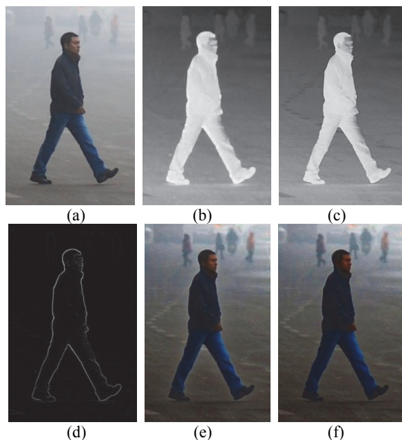
Fig. 8. Example of halation (a) Original image; (b) Transmission map estimation with 7 \times 7 mask size; (c) Transmission map estimation with 1 \times 1 mask size; (d) Results of the difference of images; (e) Halation removal without erosion method; (f) Halation removal with erosion method.
