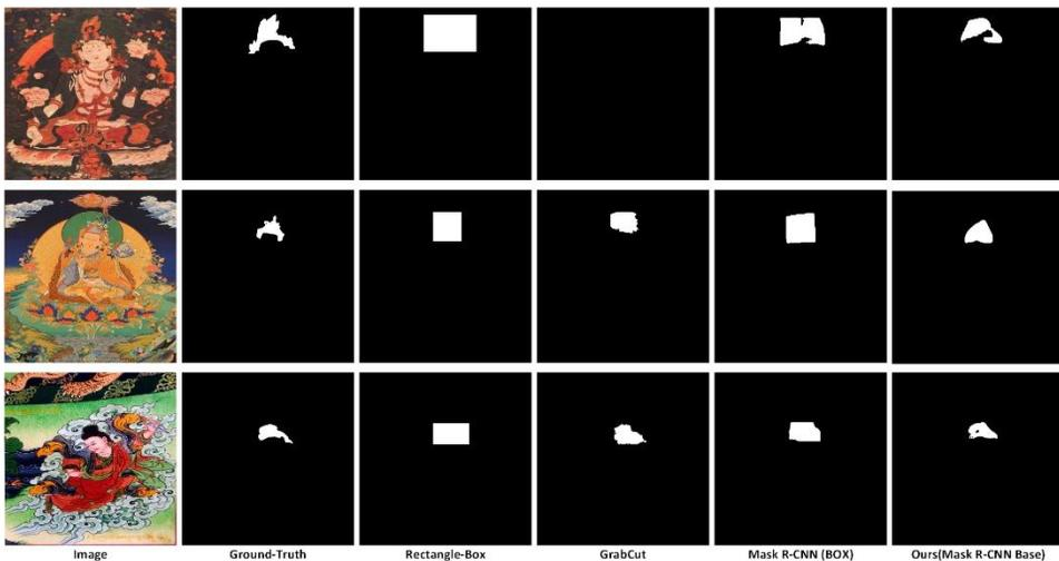
Fig. 6. Examples of the segmentation results of our approach and baseline methods. The first column is the original image. The second column is the ground-truth image. The third columns are the rectangle-box image. The following three columns show the results of GrabCut, Mask R-CNN (Box-level annotation), and proposed method (base on Mask R-CNN).
