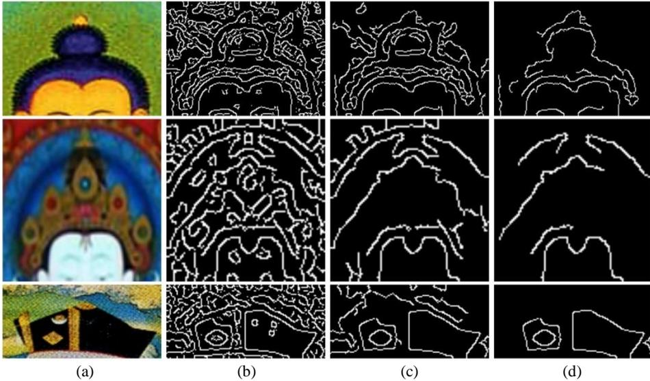
Fig. 3. The results of different values of the Canny algorithm. The first row of pictures is the chignon, the second row is the coronet, and the third row is mitral; (a) Input box images, (b)  $P \leq 0.2$ , (c)  $P \leq 0.1$ ; (d)  $P \leq 0.05$ .
