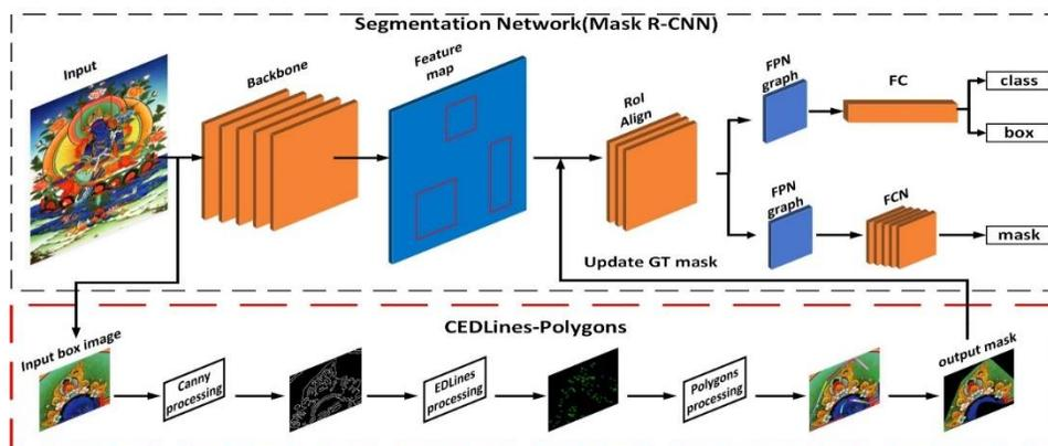
Fig. 2. The CEDLines-Polygons integrated into Mask R-CNN. The bottom part of the figure is an overview of the CEDLines-Polygons.
