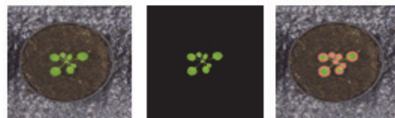
Original image Leaf extraction Leaf identification Fig. 7. Identification of Leaves in a plant image from dataset A2.
