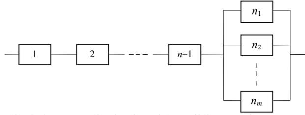
Fig. 2. Structure of a simple serial-parallel connection system.
