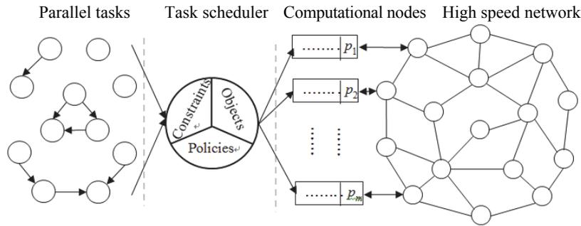
Fig. 1. A parallel computing system.
