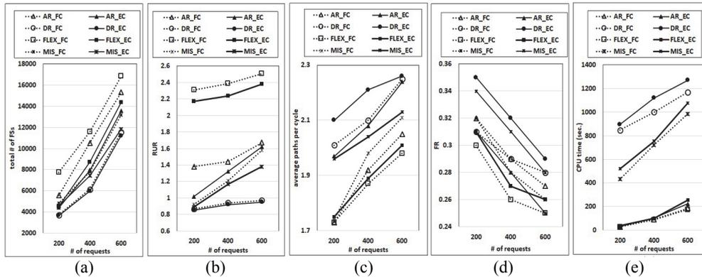
Fig. 5. Simulation results for different numbers of connection requests (a) total number of allocated FSs; (b) RUR; (c) the average number of lightpaths protected by a cycle; (d) FR; (e) CPU time in seconds.
