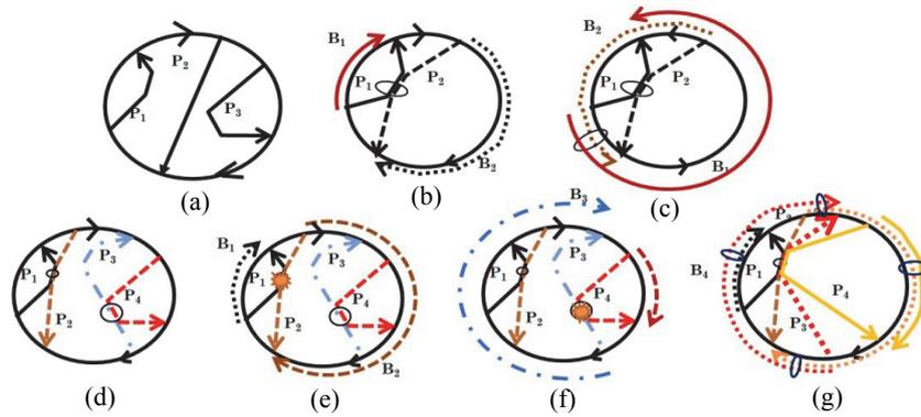
Fig. 2. Example of the problem; (a) link-disjoint lightpaths; (b) overlapped lightpaths; (c) protecting paths for (b) if common link failed; (d) more complex example; (e) protecting path for (d); (f) protecting path for (d); (g) more complex example with overlapped lightpaths.
