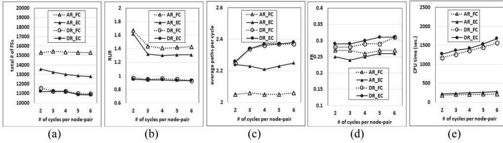
Fig. 4. Simulation results for 600 connection requests (a) total number of allocated FSs; (b) RUR; (c) the average number of lightpaths protected by a cycle, (d) FR, (e) CPU time in seconds.
