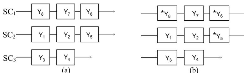
Fig. 3. (a) The scan chain architecture for s208; (b) The observing scan cell distribution for  $V_2$ .
