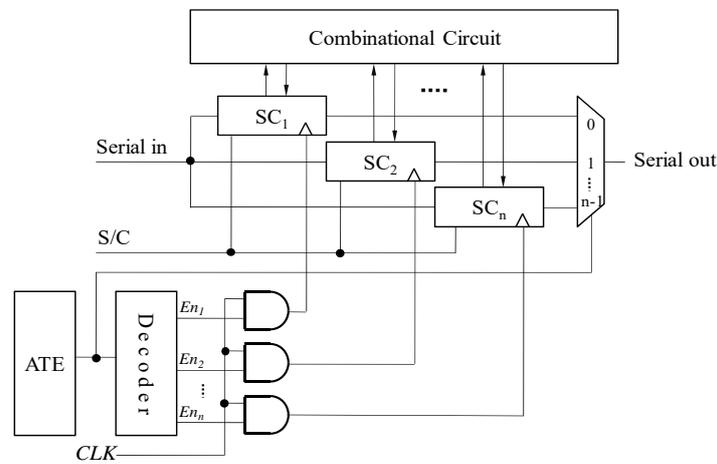
Fig. 4. Multi-scan architecture with scan chain disabling scheme.
