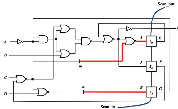
Fig. 1. An example with benchmark circuit s27.
