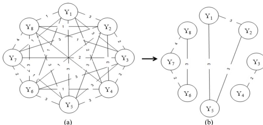
Fig. 2. (a) Weighted observability graph for s208; (b) Three cliques after partitioning.
